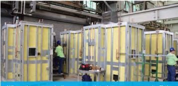
When the outer shells are completed they are moved off the leveling plates to the finishing area where the plumbing fixtures, electrical, tiling and all other is work is done to complete the bathroom pod.
